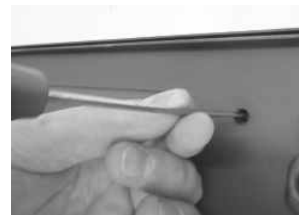
3). Remove Plastic Fixing Rivets.
