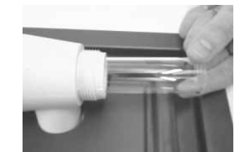
7). Carefully remove quartz sleeve
