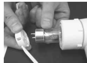
5). Disconnect lamp holders and remove lamp
